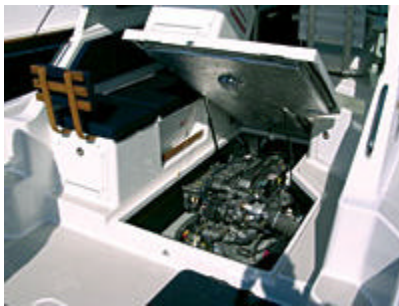
The single Yanmar 315 hp Diesel sits in a well-insulated compartment underneath the helm deck. The dinette (below) in the bow converts to a generous-sized double berth.
