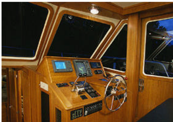
A double helm seat, a good line of sight and ample space for electronics create a functional lower helm station. While not in use, the back of the helm seat folds down, providing a counter for the bar area.
